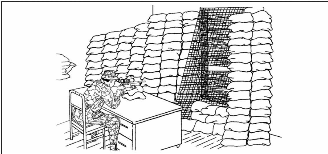
Figure 6-2. Internal View of a Room Hide
