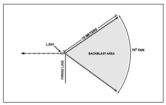
Figure B-1. M72A7 backblast area
