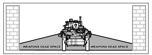
Figure B-11. Mobile gun system dead space at street level
