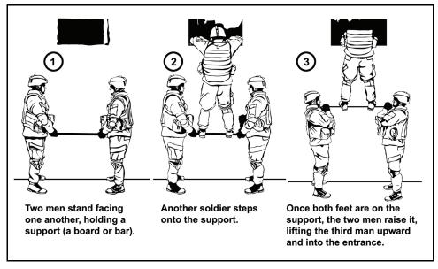
Figure 7-2. Two-man supported lift
