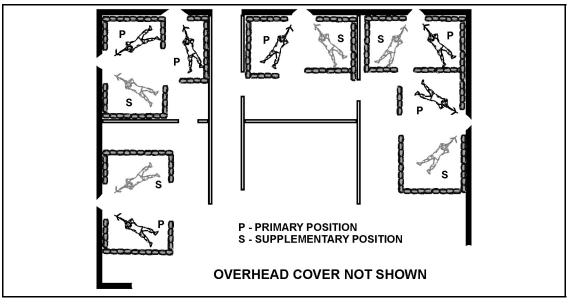
Figure 7-49. Loopholes with primary and supplementary positions
