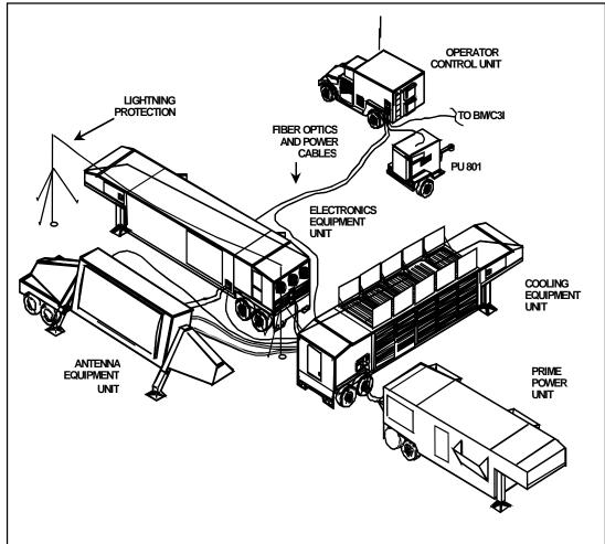
Figure 4-1. THAAD Radar Components
