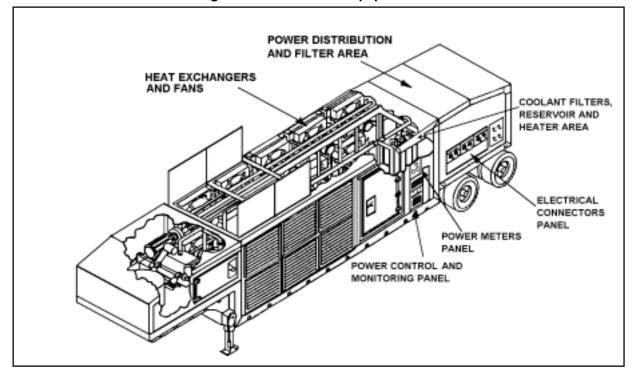
Figure 4-4. Cooling Equipment Unit
