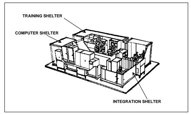
Figure 7-5. Unit Conduct of Fire Trainer
