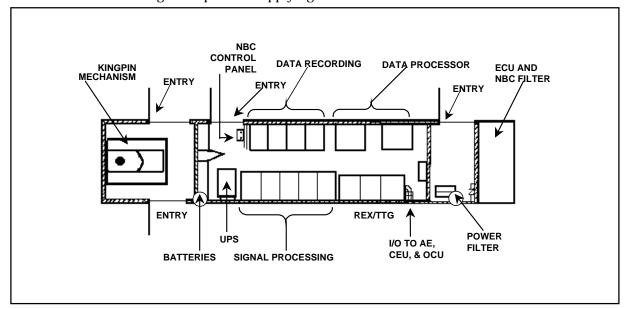
Figure 4-3. Electronics Equipment Unit
