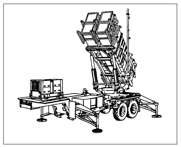
Figure 5-6. Launching Station Emplaced (PAC-2)
