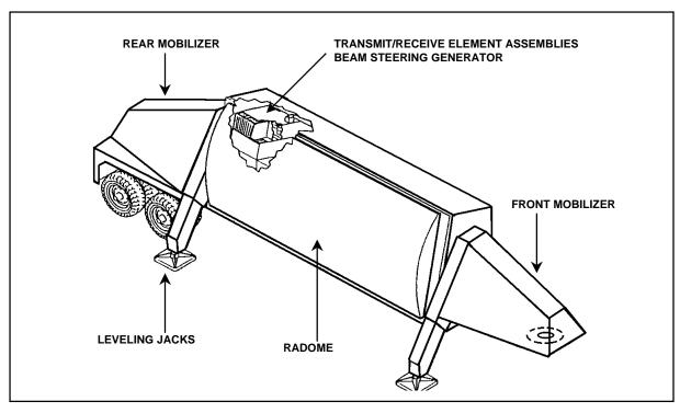
Figure 4-2. THAAD Antenna Equipment Unit
