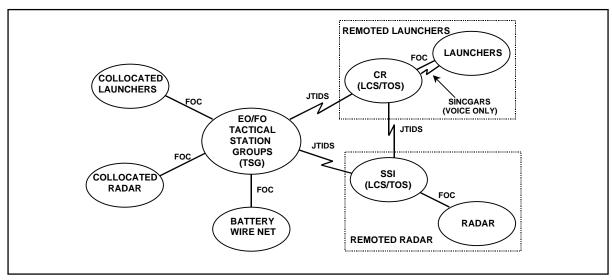
Figure 4-10. Battery Mission Operations Net
